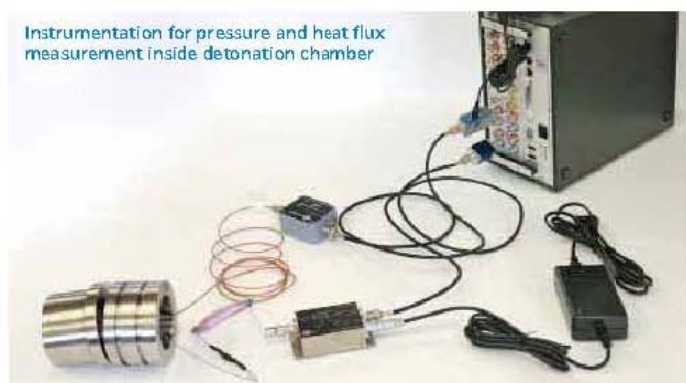
Pressure and coaxial thermocouple record from detonation chamber KV-250
